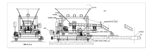
Fig: Vibratory charge system for double trolley cross & lateral travel.
